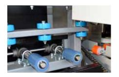
The transmission is made by hard nylon reinforced with glass fiber conical pinions, Teflon core with Vulkollan external layer geared rolls and stainless steel shafts, which means: low noise level, no need to lubricate, low maintenance, no corrosion and safety for operators.
