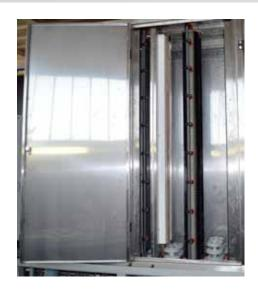
Machine body, including all doors, spraying bars (on request) & water tanks are completely made of Stainless Steel, this means:
