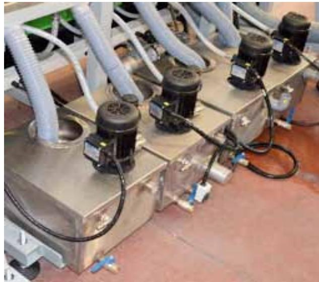
Machine body and water tanks are completely made of Stainless Steel, this means: no corrosion, high quality machine and longer lifetime.
