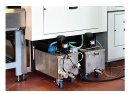
Water tanks with pumps and filters are easy extractible, moving on wheels. Stainless steel extractible drawers for glass scrap recovery.
